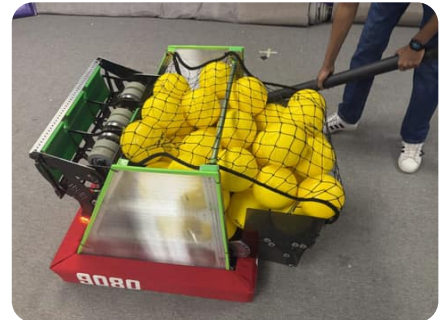
55 ball capacity big dumper archetype side view
